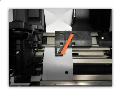
The paper is aligned to the left and the sensor mirror, which is located on top, has to be adjusted as central as possible to the paper in order to detect the perforation of the green fee tickets and pull back and cut the ticket.
