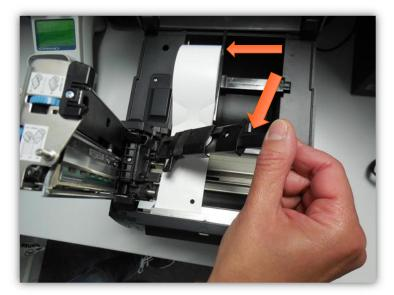
Pull this lever up as well by pressing the lateral button to get to the paper layer. It is now possible to replace the paper roll. Make sure to insert the new roll correctly with the white side, which is to be printed, facing upwards.
