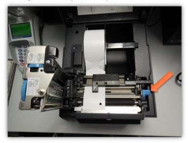
At first, open the thermal printing head by pressing the release lever on the right-hand side of the printer.
